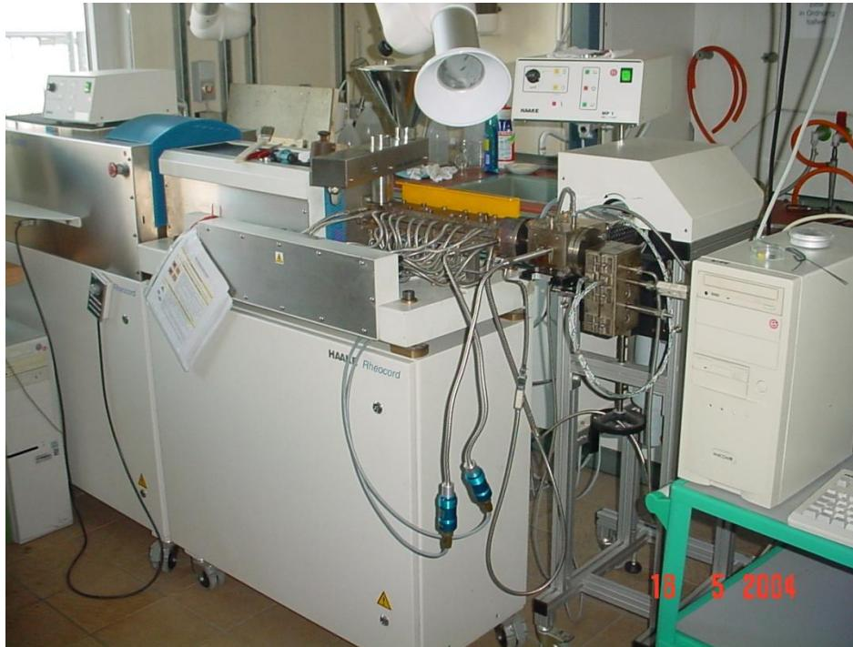
**Figure 20.1 Mini-Twin-screw-extruder** for sample-production in lager scale (500 g / h)
