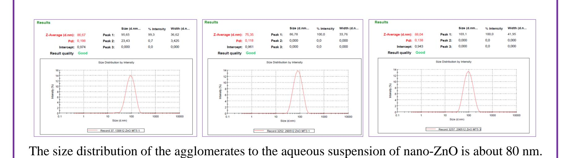
Agglomerate size as measured by DLS analyzer (Malvern, model Zetasizer-ZS).
