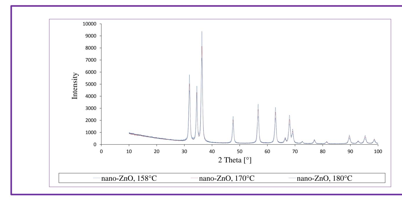
X-ray diffraction results of the obtained nano-ZnO. It is possible to obtain nano-ZnO at a temperature of about 160°C.
