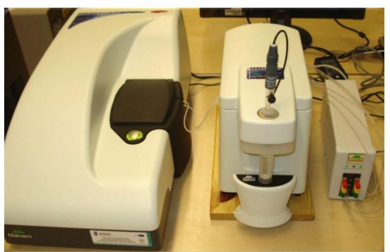
The **Zetasizer Nano ZS** is a high performance two angle particle and molecular size analyzer for the enhanced detection of aggregates and measurement of small or dilute samples, and samples at very low or high concentration using dynamic light scattering with 'NIBS' optics. The ZSP also incorporates a zeta potential analyzer that uses electrophoretic light scattering for particles, molecules and surfaces, and a molecular weight analyzer using static light scattering.
