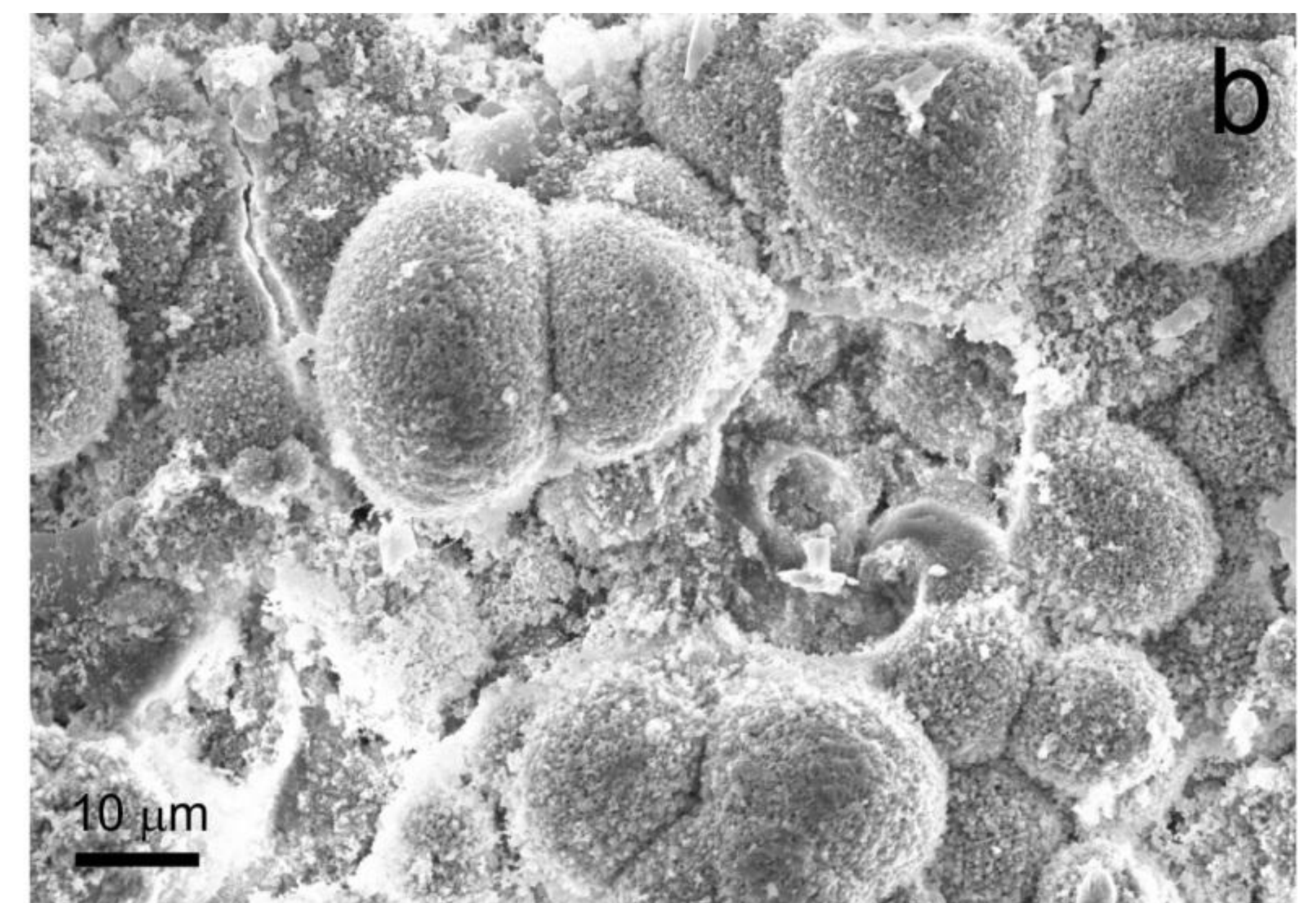
Surface of the nano-Ti-6Zr-4Nb after anodic oxidation (a) and additional Ca-P deposition (b).
