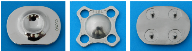
Fig. 3. INOP/LSL.1101 endoprosthesis components made of various materials with the use of various technologies, the condition of surface after polishing: a) upper plate, CoCrMo alloy, CNC machining, b) insert, 316L steel, CNC machining following gear forging, c) bottom plate, Ti6Al4V alloy, SLM technology
