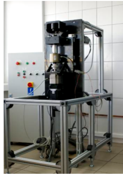
4. A view of the simulator for the testing of spine implants [4, 5]
