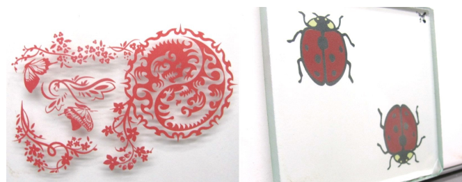
Fig. 3. Examples of laser decoration of glass plates from Ceramika Tubądzin.
