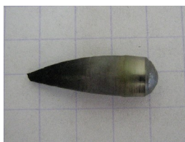
Fig. 2. A single crystal of \text{Ce}_2\text{IrSi}_3 grown by Czochralski technique in the tetra-arc furnace.
