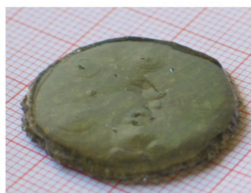
Fig. 1 Multi nucleation during the hetero-epitaxial growth of an AlN single crystal on C-face SiC substrate
