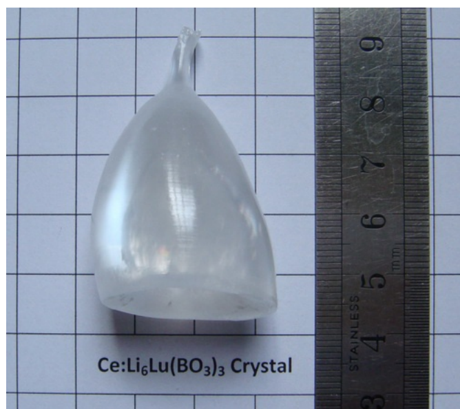
Fig 1. As-grown crystal of Ce:Li 6 Lu(BO 3 ) 3 grown by the Czochralski technique
