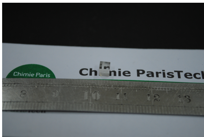
Fig. 1: YAB single crystal cut in the ZX plane for 266 nm generation [1]X. Yu et al, Journal of Crystal Growth, 312, 3029–3033 (2010) [2]J. Yu et al, Journal of Crystal Growth, 341, 61-65 (2012) [3]H. Liu et al, Materials Research Innovations, 15, 102-106 (2011)
