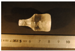
Fig. 1: CBF single crystal grown using LiF as a flux
