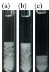
Fig. 1 Crystals images in three types of solutions at T_1 and t = 495 hrs. (a) 5 components, (b) 3 components (c) 2 components.
