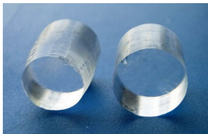
Photograph of SR grown ammonium acid phthalate crystal
