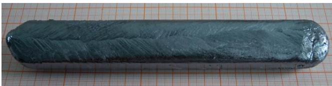
Fig.1 The synthesized ZnGeP 2 polycrystalline ingots with 470g
