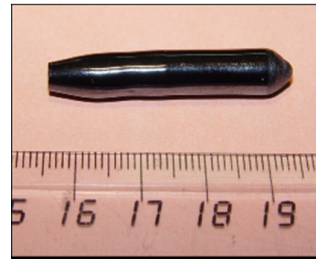
Fig.1 As grown GaFeO_3 single crystal
