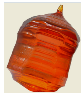
Fig. 2 4 inches Langasite crystal growth along Euler angles (0°, 138.5°, 26.7°)
