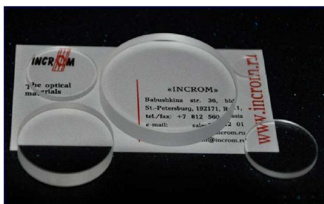
Fig.1. \text{CaF}_2:\text{Yb} laser ceramics
