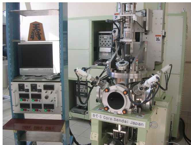
Fig. 1. The tetra-arc Czochralski furnace installed at the Institute of Low Temperature and Structure Research, Polish Academy of Sciences in Wrocław.
