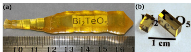
Figure 3 - (a) As-grown BTeO crystal using de double crucible method; (b) Polished samples used for the optical measurements.
