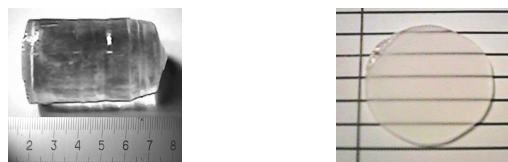
Fig.1. Li 2 MoO 4 single crystal grown by Czochralski technique and Ø25x1 mm plate cut from the crystal
