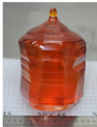
Fig. 1 4 inches Langasite crystal growth along Euler angles (0°, 22°, 90°)
