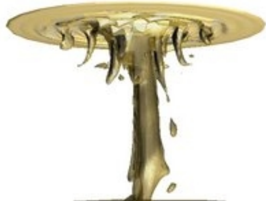
Fig. 5. The spatial picture of thermics under the disk in 3D-calculation, which has been plotted as isothermal surface at T = 312 K.
