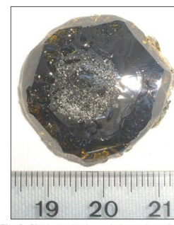
Fig. 2 Single nucleation spiral growth mode of an AlN single crystal on C-face SiC substrate
