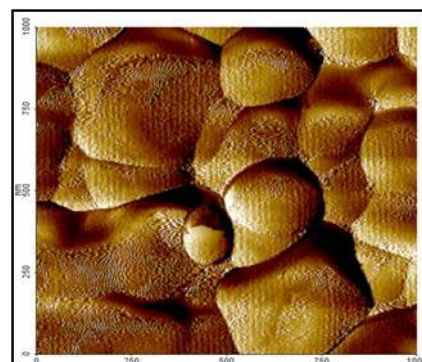
Figure 1: MFM image of the Li,Co codoped film over scan area of 1000 nm \times 1000 nm. References: 1. U. Ozgur, Ya. I. Alivov, C. Liu, A. Teke, M. A. Reshchikov, S. Dogan, V. Avrutin, S.J. Cho, and H. Morkoc, J. Appl. Phys. 98 , (2005) 041301 2. M. Venkatesan, C. B. Fitzgerald, J. G. Lunney and J. M. D. Coey, Phys. Rev. Lett. 93 (2004) 177206.
