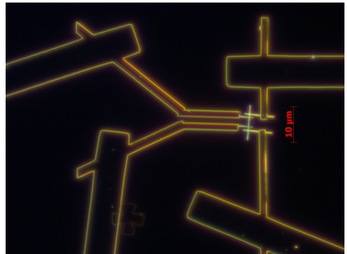
Figure 1: SEM picture of Au-catalysed (In,Ga)As-(Ga,Mn)As core-shell nanowires grown on GaAs(111)B substrate (upper panel); magnetic properties of nanowires ensemble (middle panel); optical image in dark field of isolated nanowire on Si/SiO 2 substrate contacted to four terminals by e-lithographic methods (lower panel).
