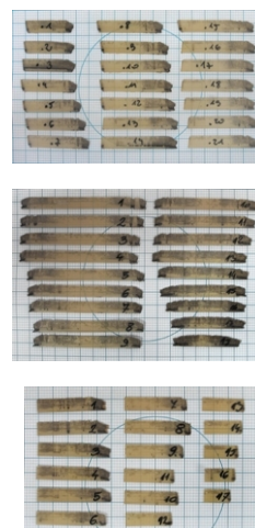
Fig. 2. Stripes sliced from the HVPE-GaN boule with various exposed surfaces: a) (20-21); b) (10-10); c) (11-20); grid line 1 mm.
